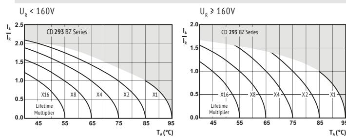
$I_A$  = actual ripple current at 120Hz,
