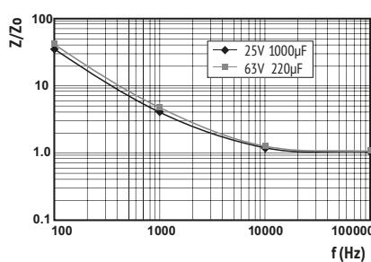
$Z =$  actual impedance of each frequency at  $20^\circ C$ ,
