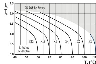
$I_A$  = actual ripple current at 100kHz,
