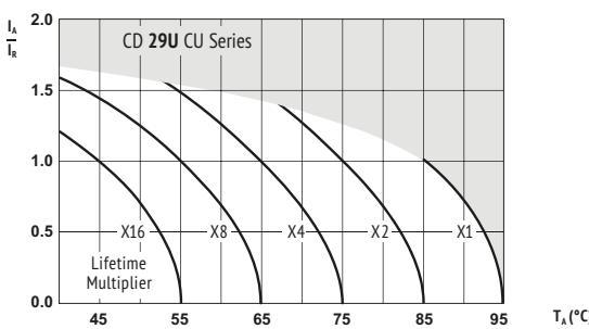
$I_A$  = actual ripple current at 120Hz,
