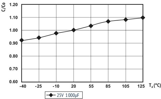
$C$  = actual capacitance of each temperature at 100Hz,
