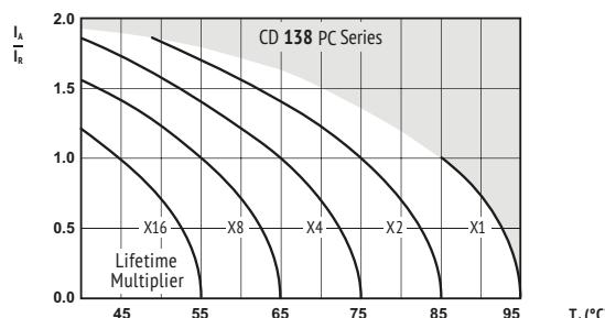
$I_A$  = actual ripple current at 120Hz,
