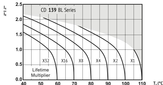
$I_A$  = actual ripple current at 120Hz,
