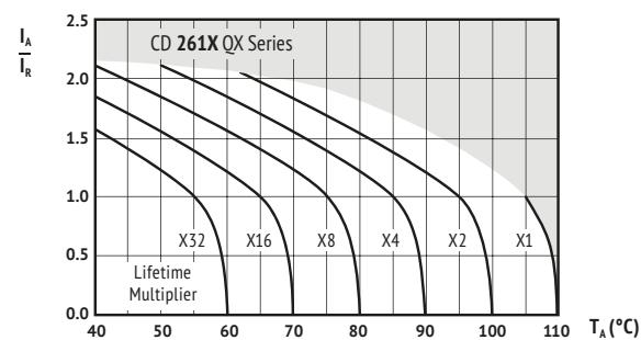
$I_A$  = actual ripple current at 100kHz,
