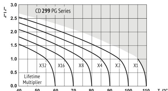
$I_A$  = actual ripple current at 120Hz,
