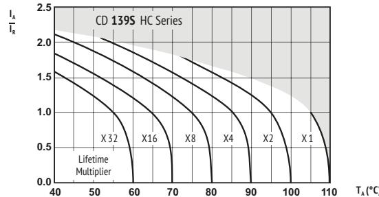
$I_A$  = actual ripple current at 120Hz,
