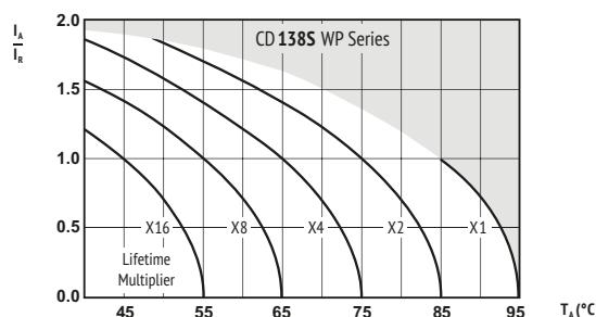
$I_A$  = actual ripple current at 120Hz,
