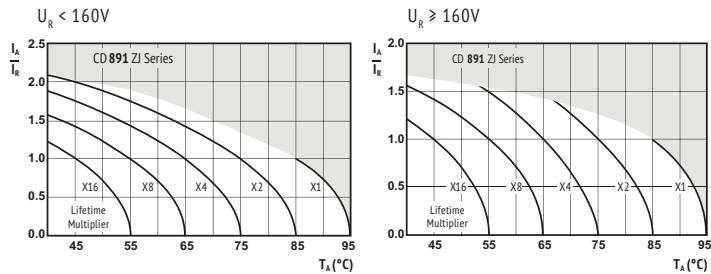
$I_A$  = actual ripple current at 120Hz,
