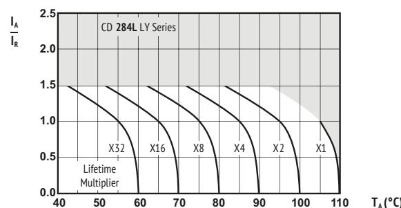
$I_A$  = actual ripple current at 100kHz,
