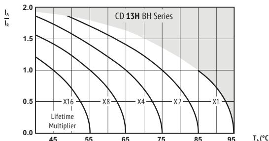
$I_A$  = actual ripple current at 120Hz,
