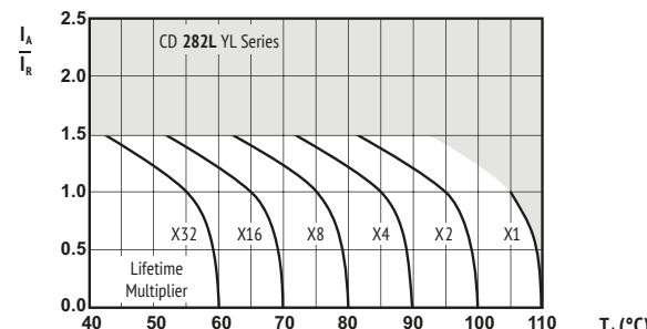
$I_A$  = actual ripple current at 100kHz,
