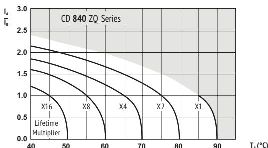
$I_A$  = actual ripple current at 120Hz,
