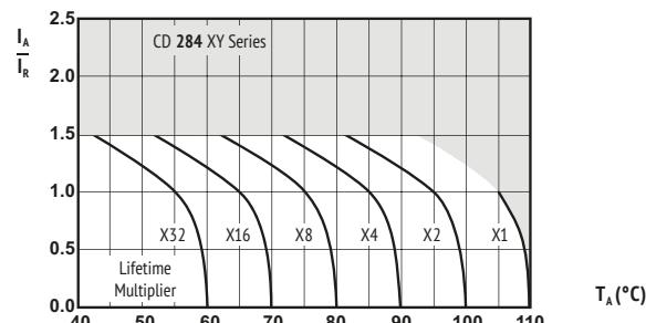
$I_A$  = actual ripple current at 100kHz,
