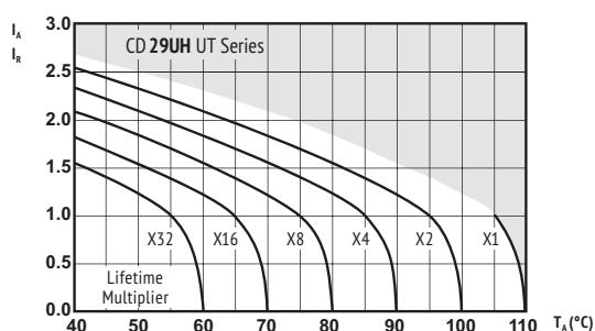
$I_A =$  actual ripple current at 120Hz,
