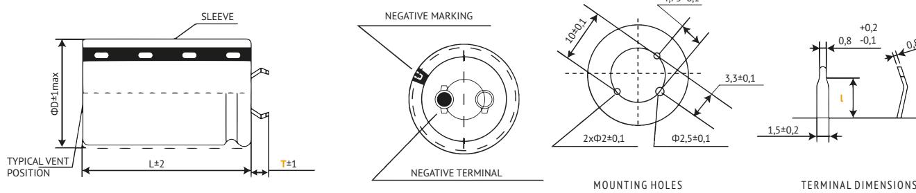
For diameter  $\phi D \geq 45\text{mm}$  the safety vent is typically placed at the side of the housing.
