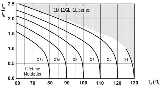
$I_A$  = actual ripple current at 120Hz, $I_R$  = rated ripple current at 120Hz, 125°C
