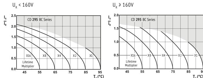
I<sub>A</sub> = actual ripple current at 120Hz,
