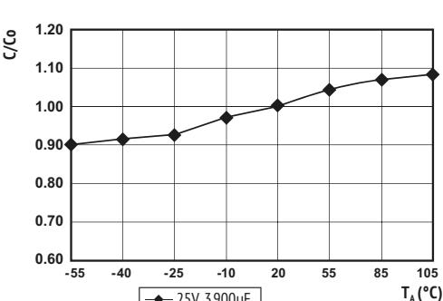
$C =$  actual capacitance of each temperature at  $100Hz$ ,
