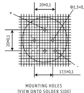
MOUNTING HOLES (VIEW ONTO SOLDER SIDE)
