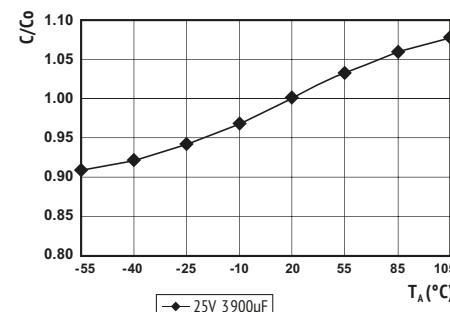
$C$  = actual capacitance of each temperature at 100Hz,
