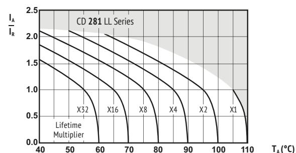
$I_A$  = actual ripple current at 100kHz,
