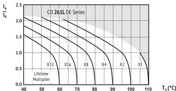
$I_A$  = actual ripple current at 100kHz,
