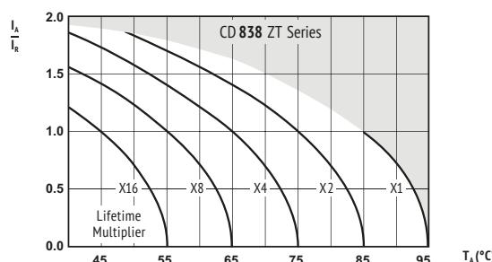
$I_A$  = actual ripple current at 120Hz,
