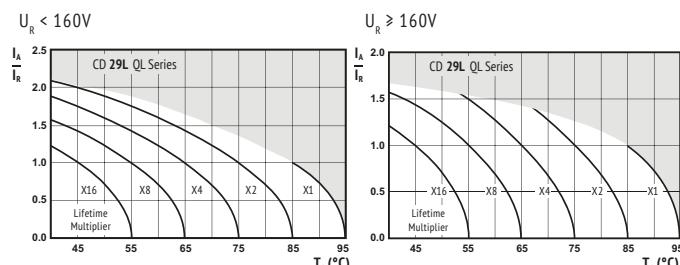
$I_A$  = actual ripple current at 120Hz,
