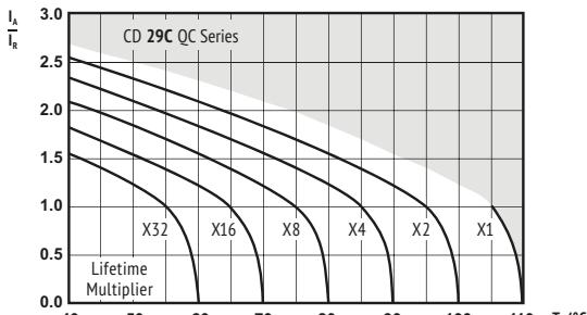
$I_R$  = actual ripple current at 120Hz,
