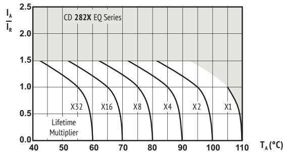
$I_A$  = actual ripple current at 100kHz,
