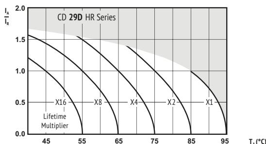
$I_A$  = actual ripple current at 120Hz,
