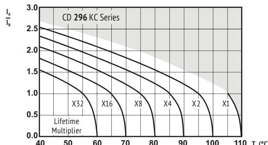
$I_A$  = actual ripple current at 120Hz
