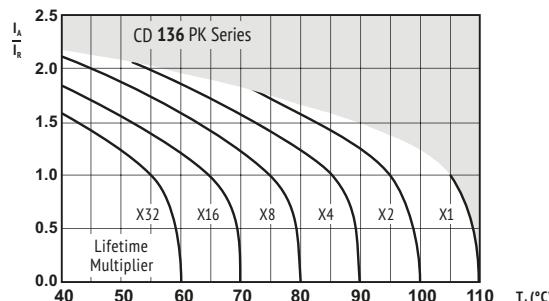
$I_A$  = actual ripple current at 120Hz,
