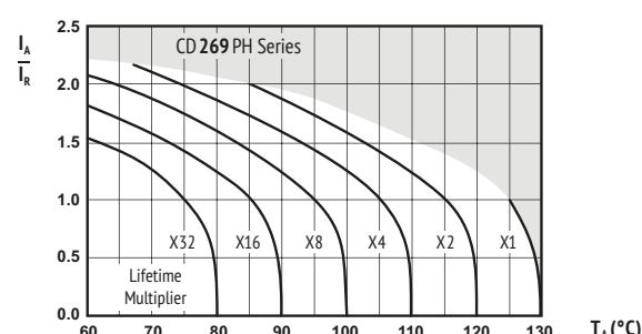
$I_A$  = actual ripple current at 100kHz,
