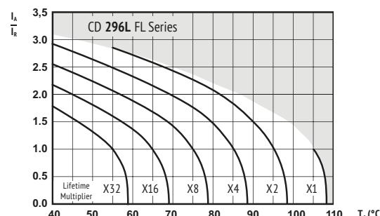
$I_A$  = actual ripple current at 120Hz,
