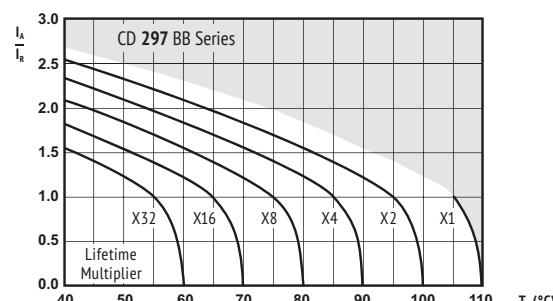
I<sub>A</sub> = actual ripple current at 120Hz,
