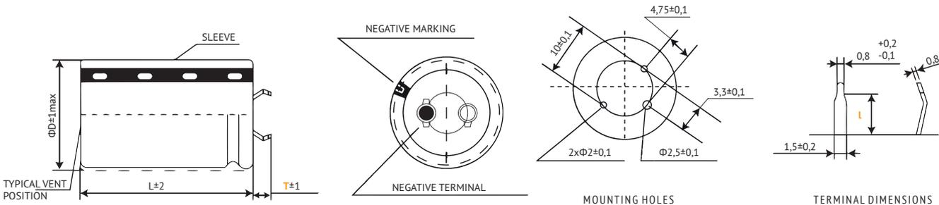
For diameter  $\varnothing D \geq 45 \text{ mm}$  the safety vent is typically placed at the side of the housing.
