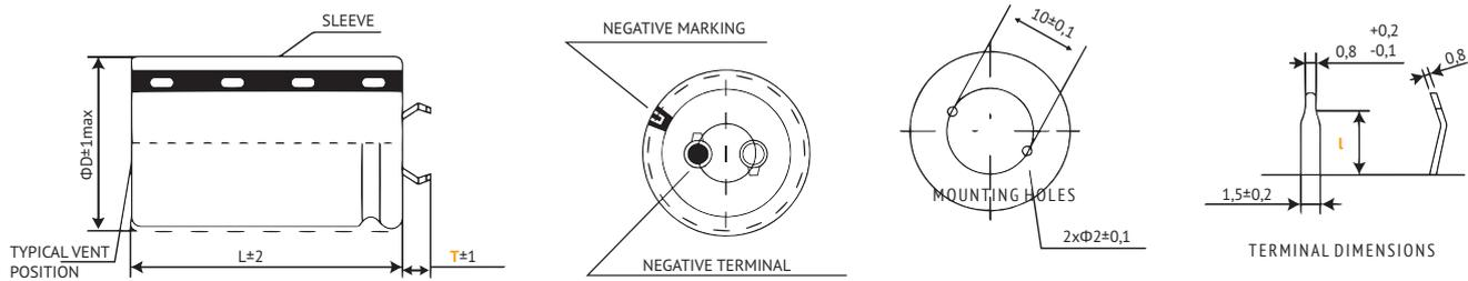
Standard version: Self-Lock Terminal. Other terminal types and styles on request. For diameter  $\varnothing D \geq 45 \text{ mm}$  the safety vent is typically placed at the side of the housing.
